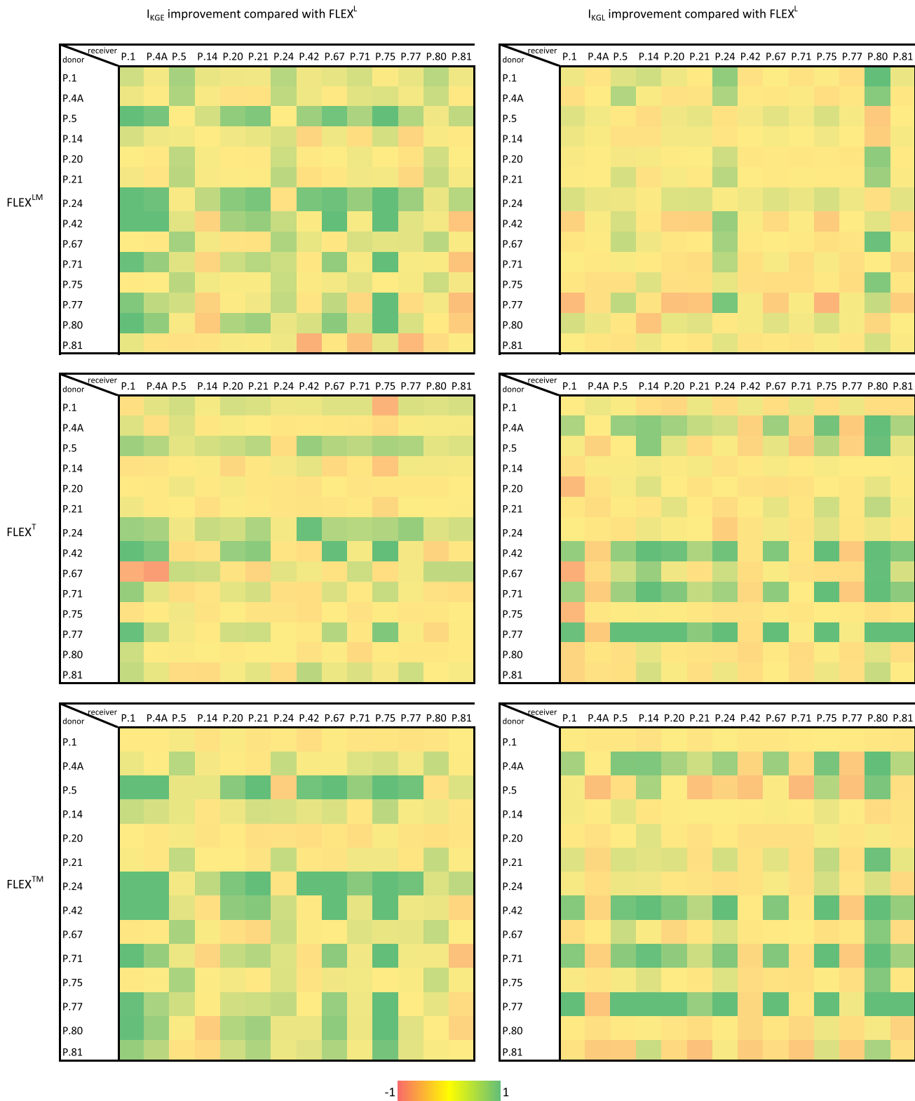
Figure 6. The improvement of three hydrological models (FLEX LM , FLEX T , and FLEX TM ) compared with FLEX L for the two calibration objective functions ( I_{KGE} , I_{KGL} ) after model transfer from donor to receiver catchments in 14 catchments. The values of objective functions are based on the mean value of each objective function from the set of Pareto-optimal solutions. Shades of green indicate slight (light green) to strong (darker green) improvement in terms of mean I_{KGE} and I_{KGL} , respectively; shades of red indicate slight (orange) to strong (red) deterioration, while yellow indicates no significant change. FLEX TM shows the best improvement for both I_{KGE} and I_{KGL} .
